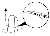
To reinstall the non-adjustable head restraint, do the following:
